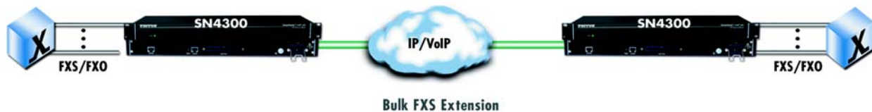
Figure 5. Bulk analog line extensions application
