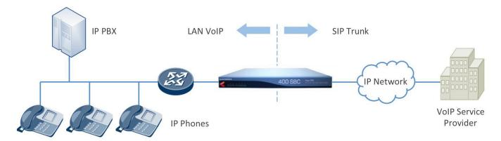
Vega SBC manages the connections between two SIP networks, for instance, between an IP-PBX and one or more ITSPs.
