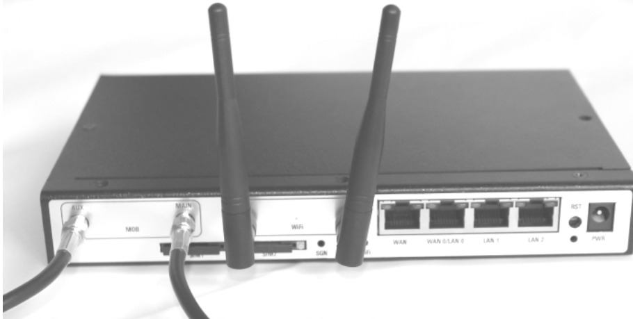
Figure 11-5: Photo of diversity-enabled Bytton, with two stick antennas for WiFi and two connectors for the 4G Mobile antennas.
