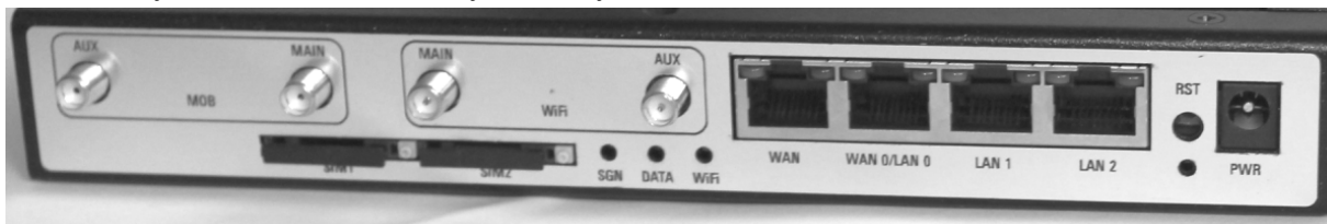
Figure 4-17: Bytton LTE with four antenna connectors, two for LTE (4G Mobile) and two for N-type WiFi access point.
