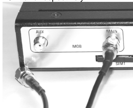
Figure 4-16: Inserting the connectors for the LTE Mobile Antennas (one or two pcs.)
