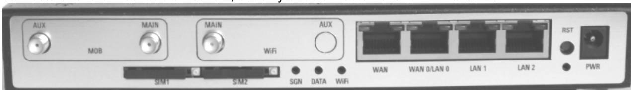
Figure 1-3: Drawing and photo of antenna diversity: up to two antennas for Mobile and Wi-Fi.
