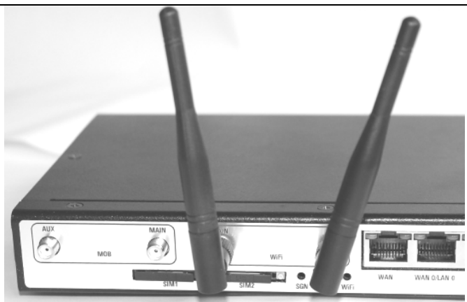
Figure 4-18: Attachment of the two WiFi Antenna for N-type wireless AP
