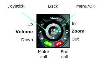
In addition to the joystick, the following buttons are available around it:
