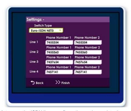
2. Select **Finish** to save the ISDN lines configuration and complete the configuration wizard.
