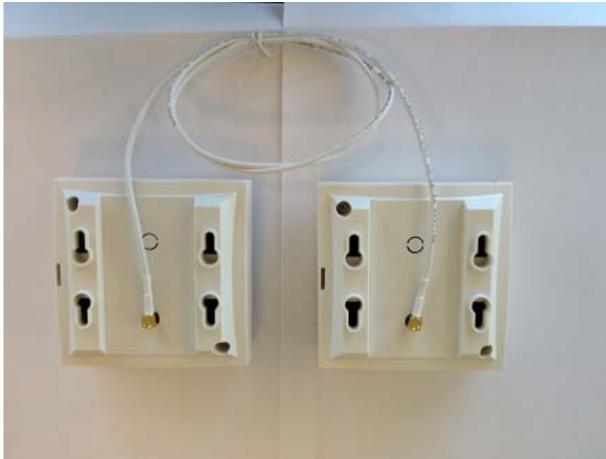
Figure 11 Connect Power to the Bottom of the Repeater and External Antenna Cable to the Rear of the Repeater
