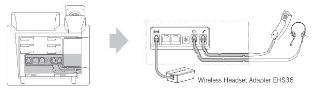
Note: The headset and wireless headset adapter EHS36 should be purchased separately. EHS36 is used for connecting the phone and a compatible wireless headset. For more information on how to use the EHS36, refer to Yealink EHS36 User Guide.
