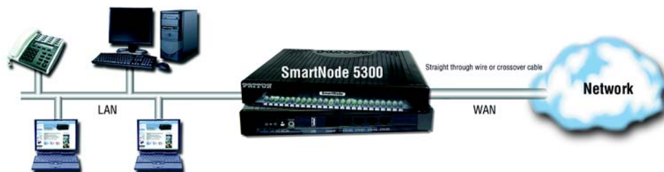
Figure 12. Connecting the SmartNode to the network
