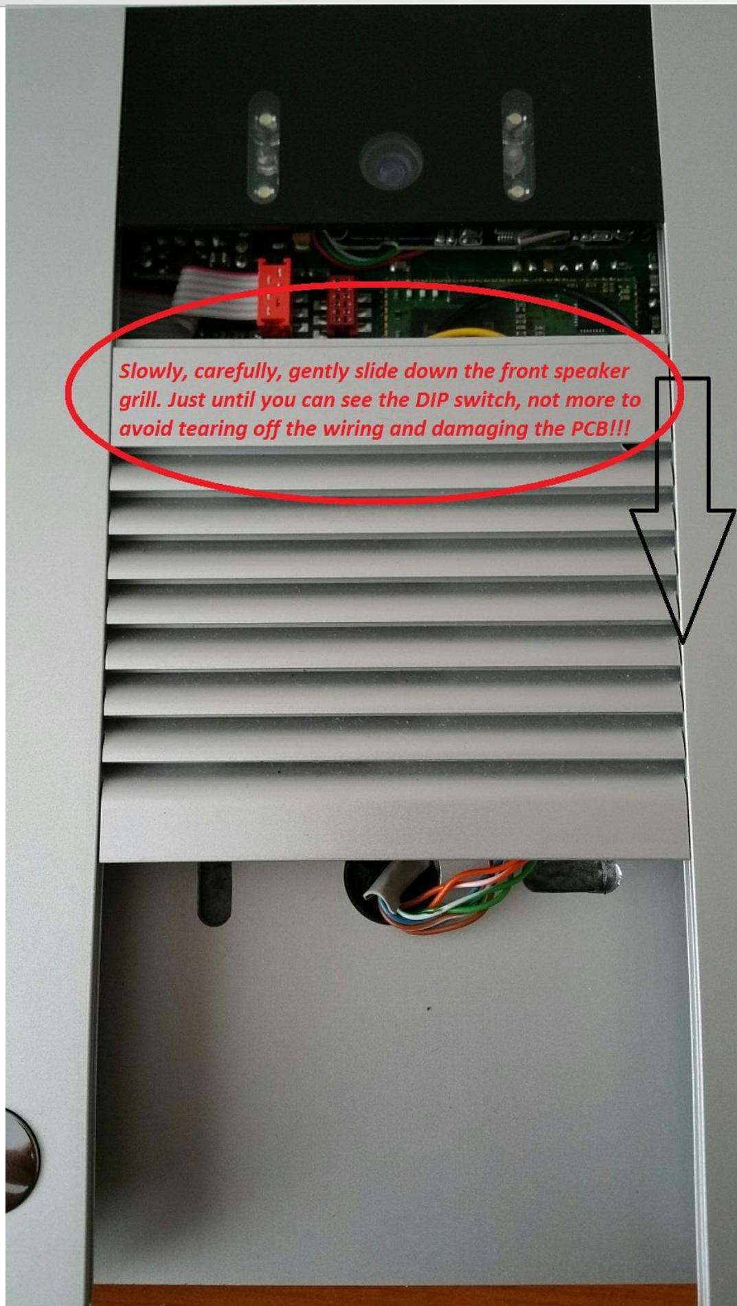
*Slowly, carefully, gently slide down the front speaker grill. Just until you can see the DIP switch, not more to avoid tearing off the wiring and damaging the PCB!!!*
