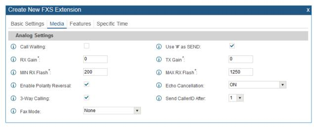
Figure 154: Configure Extension for Fax Machine: Analog Settings
