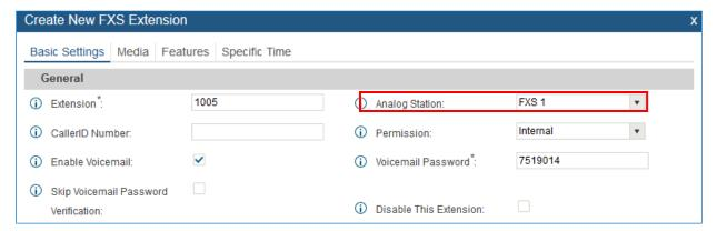
Figure 153: Configure Extension for Fax Machine: FXS Extension
