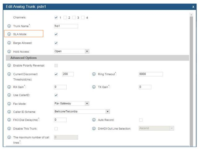
Figure 114: Enable SLA Mode for Analog Trunk
