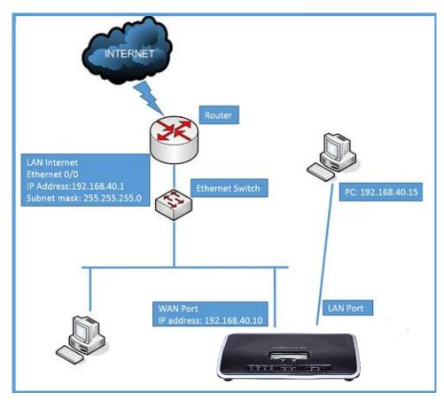
Figure 24: UCM6200 Network Interface Method: Switch
