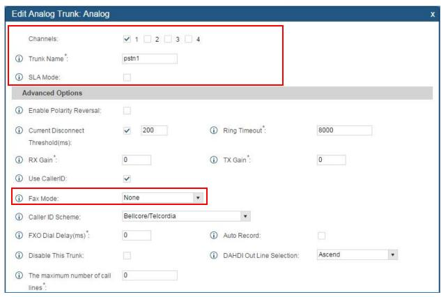
Figure 152: Configure Analog Trunk without Fax Detection
