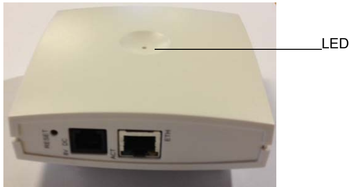
Figure 5 Base Station - Front view
