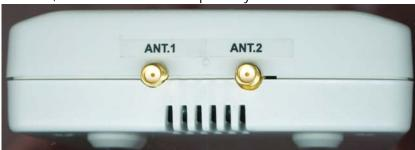
These correspond to networks Mobile 1 and Mobile 2. The cable for each Mobile antenna must be threaded into the circular connector of MobiLinkIP labeled "ANT1", respectively "ANT2", as shown in the following drawing.
