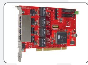
With the BN2S0, BN4S0 and the BN8S0 BRI ISDN cards, beroNet provides a powerful and flexible solution for the open source PBX Asterisk. Together with our channel-driver "chan\_mISDN", which is covered by the GPL licensing agreement, you can easily add BRI ports to your Asterisk system. Our channel-driver is based on the new ISDN stack of the new Linux Kernel: mISDN (modular ISDN).
