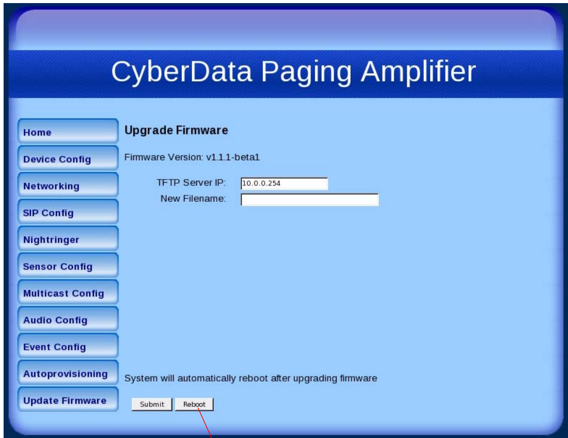
Figure 2-33. Reboot System Section
