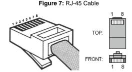
When connecting an Ethernet cable to the Mediatrix 4400, use a standard telecommunication cord with a minimum of 26 AWG wire size. It is possible to use either a crossover or straight Ethernet cable to connect in the Ethernet connectors. These connectors perform automatic MDI / MDIX detection, meaning that they adapt to the type of cable connected to them.
