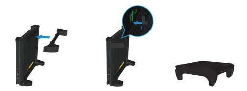
Place the locking catches of the mounting stand into their slots on the Technicolor Gateway and slide the mountable stand into place.
